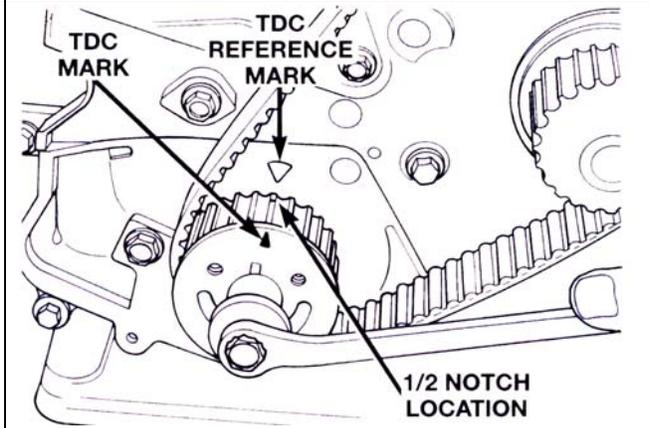
**Fig. 8: Aligning Crank to the 1/2 Mark**
