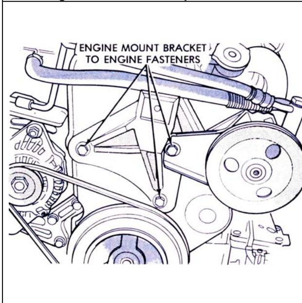
**Fig 3: Engine Mount Removal**
