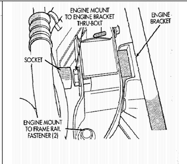
**Fig 2: Right Engine Mount Removal**
