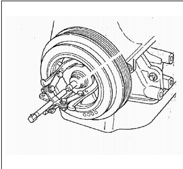
**Fig 1: Crankshaft Damper Removal**
