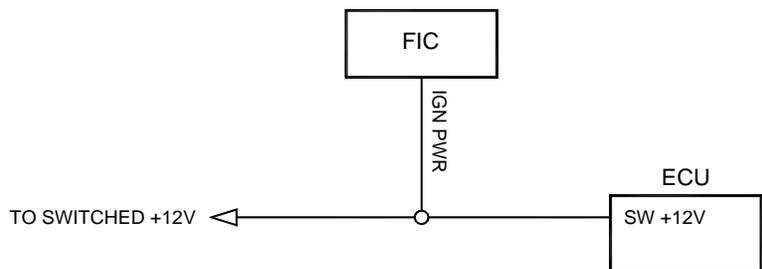
Figure 17: F/IC power connection
