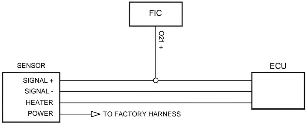
Figure 15: Current sync O2 sensor connection
