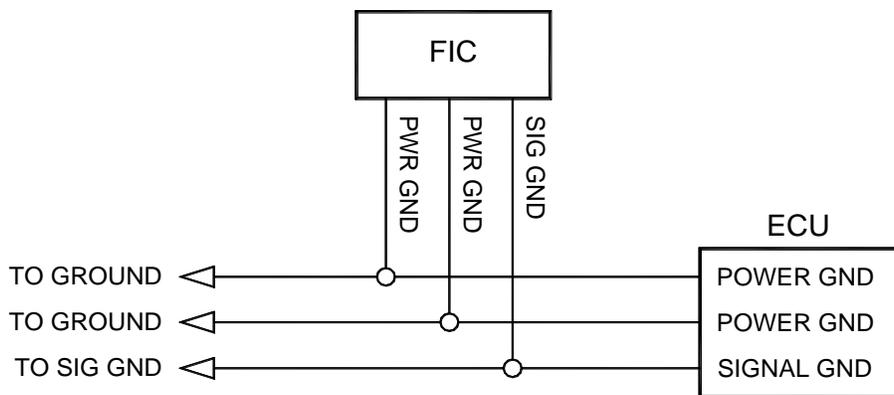
Figure 19: Power ground connections
