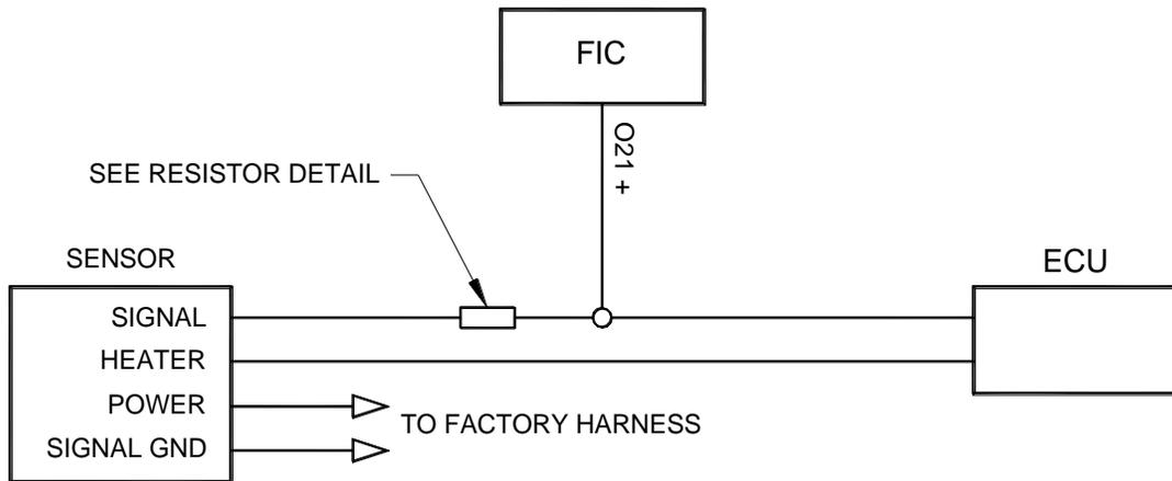
Figure 13: Narrowband O2 sensor connection
