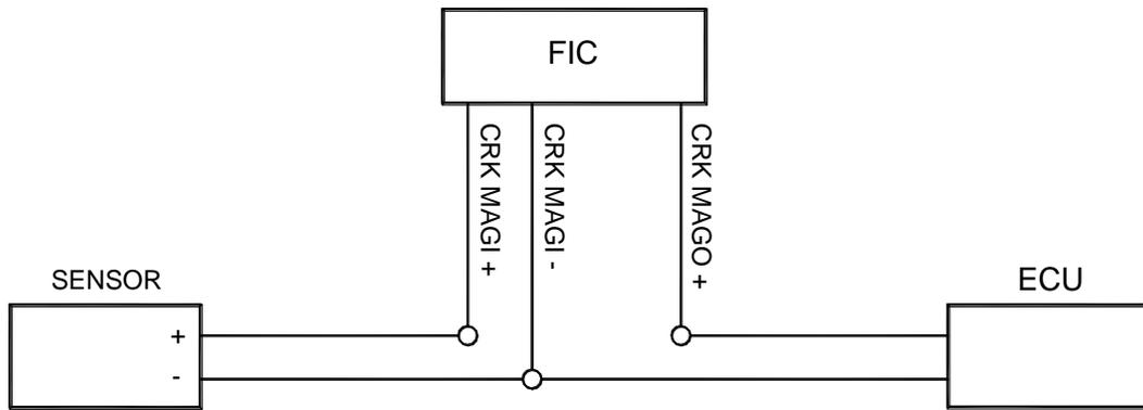
Figure 4: Crank Mag connection
