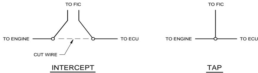
Figure 2: Wire connections
