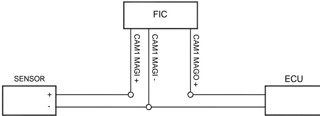
Figure 6: Cam 1 Mag connection
