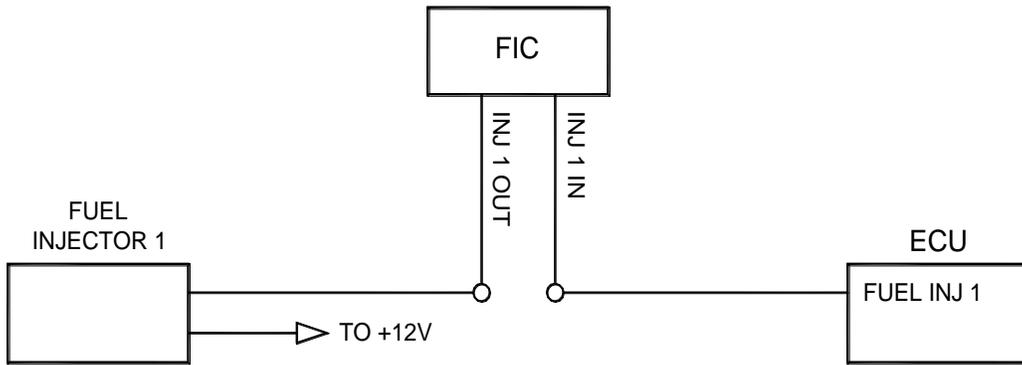
Figure 11: Primary fuel injector connection
