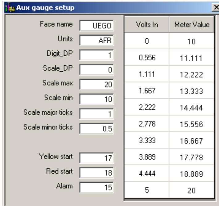
Figure 42: Auxiliary gauge setup
