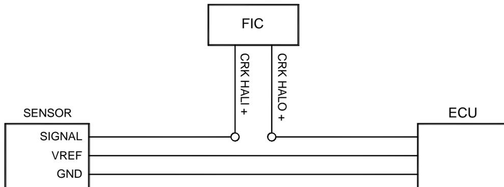
Figure 3: Crank Hall connection
