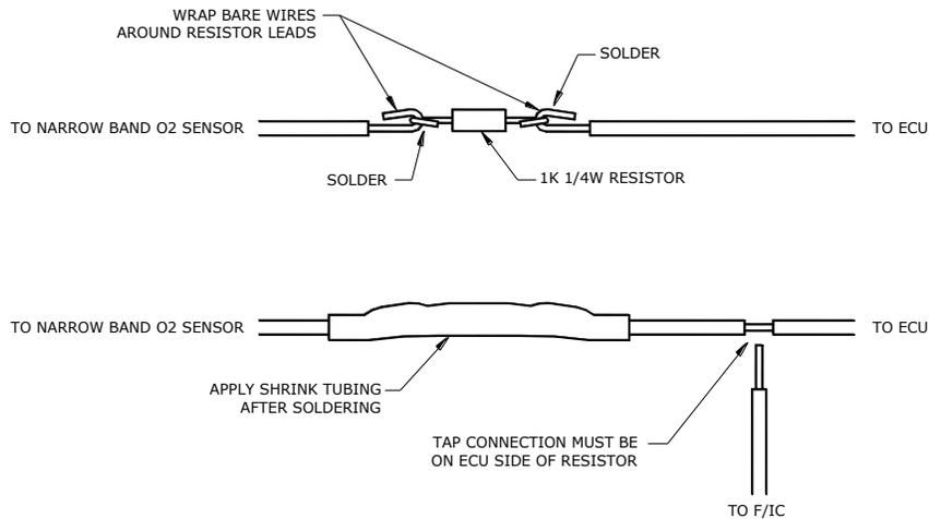
Figure 14: 1K resistor detail for narrowband O2 sensor
