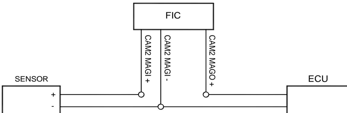
Figure 8: Cam 2 Mag connection
