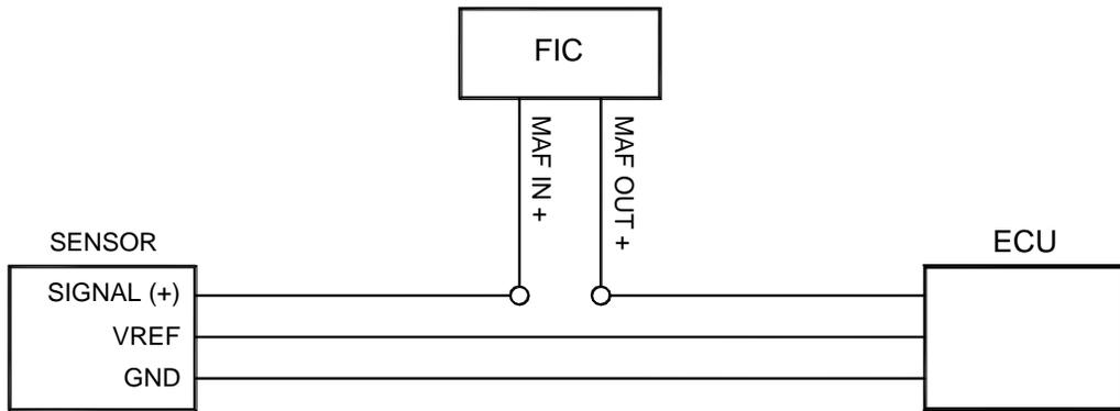
Figure 9: MAF sensor connection
