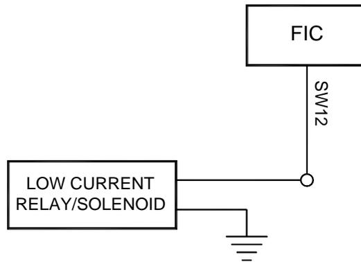
Figure 20: Switched 12V<sub>DC</sub> connection
