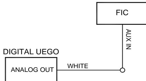
Figure 22: Digital UEGO gauge connection
