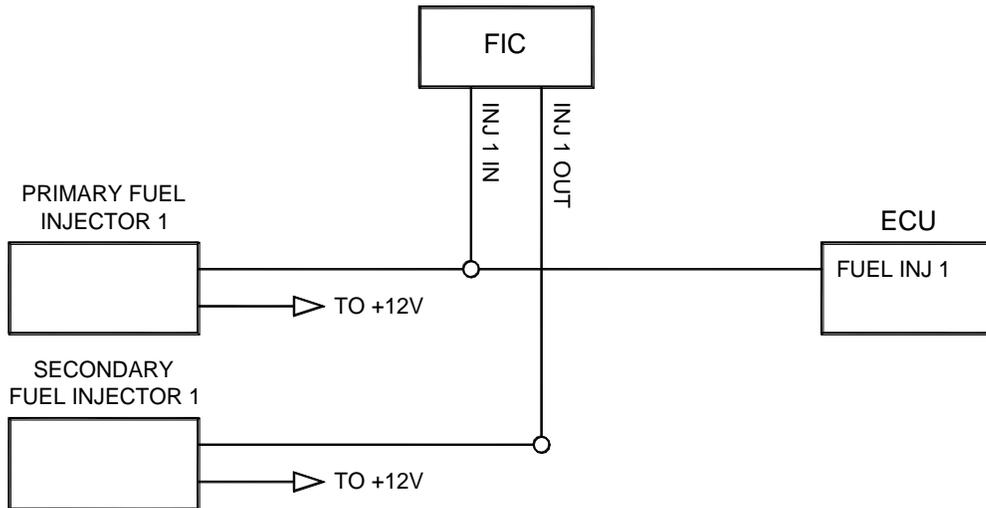
Figure 12: Secondary fuel injector connection
