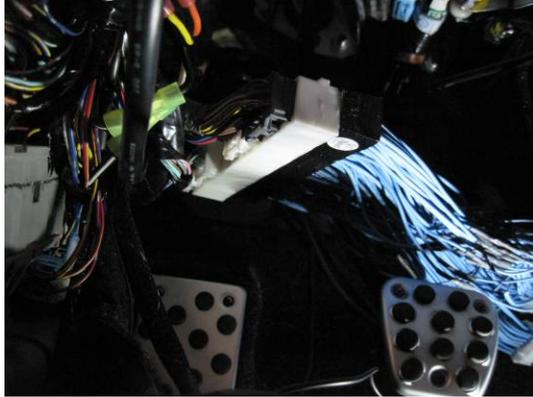
Plug in adapter harness to stock wiring
